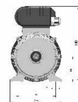
Frame with feet and end-shield with flange (IM B3)
