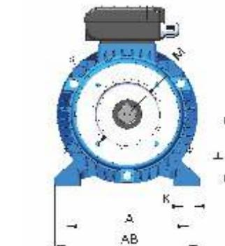
**Frame with feet and end-shield with flange (IM B34)**
